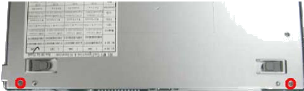
Fig. 13 Removing the screws retaining the LCD Module
